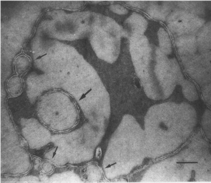
FIG. 5. Cross section of a wool fiber with interpenetrating cortex cells (TEM), bar = 200 \mu\text{m} [9].
